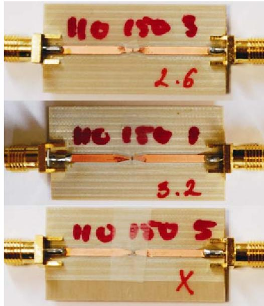
Fig. 1. Tapered microstrip line structures with a 0.15 mm gap covered with exfoliated graphene layers.
