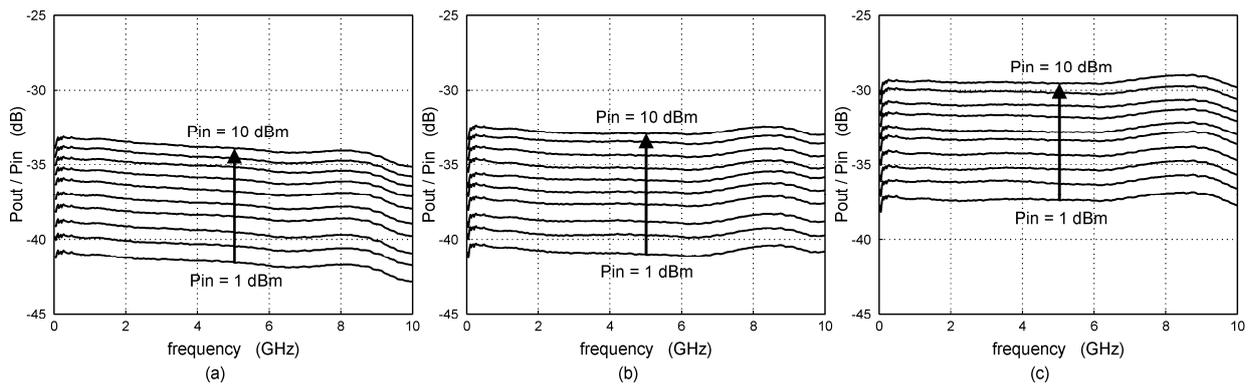
Fig. 2. Relation between the provided input power  $P_{in}$  at the fundamental frequency  $f_0$  and the measured output power  $P_{out}$  at the third harmonic component at  $3f_0$ , for three types of graphites with corresponding angular spread of the crystallite  $c$ -axes: (a) 2.6°, (b) 3.2°, and (c) less oriented graphite.
